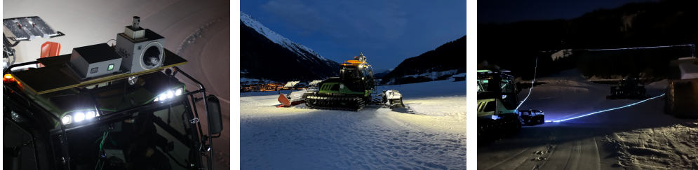
Figure 3: (Left) Our prototype is mounted atop a snow groomer. (Middle) Side view of the test vehicle. (Right) Field-of-View (FOV) outlined by the laser projector.
