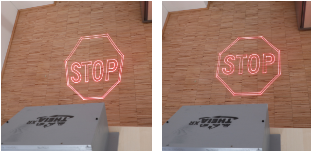
Figure 4: (Left) A projected STOP sign appears distorted from the laser’s viewpoint after tilting the projector roughly 45^\circ . (Right) The same sign appears undistorted after applying our oblique projection workflow.
