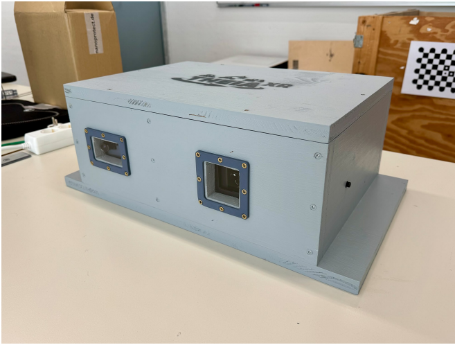
Figure 5: (Left) Image of the proposed prototype with the camera aperture on the left sight and the aperture for the laser projector on the right side. The baseline between both devices is 23 cm. (Right) Open prototype showing the internal components.
